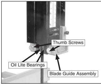
Figure 55. Front of upper blade guide.
